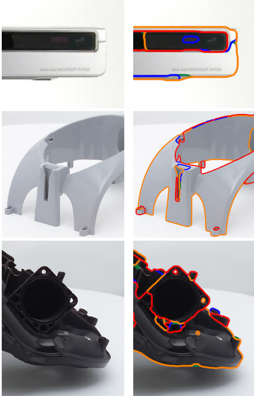
Figure 4.4: The images are taken in the photo studio. The objects are commercial products, the first row is a part of DVD player and the others are parts of a component in a machine. Even though the objects are taken on the simple background, there are well-known difficulties in image segmentation: the weak edge and complexity of shapes such as holes and multiple junctions. Note that weak edges are shown in the right side of DVD in the first row and the bottom of the object in the last row. The proposed model clearly captures boundaries of objects.
