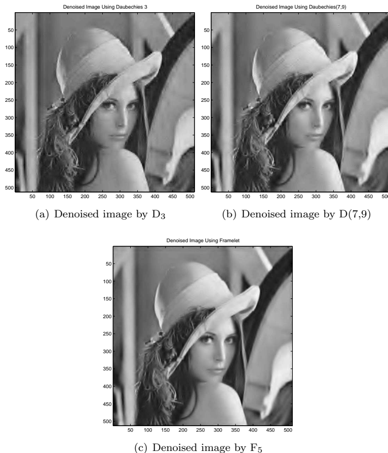
Fig. 10. The denoised images with the threshold 50, 50, and 35 by D_3 , D(7,9) , and F_5 , respectively.
