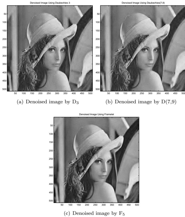
Fig. 8. The denoised images of the highest PSNR's with the threshold 30, 30, and 20 by D_3 , D(7,9) , and F_5 , respectively.
